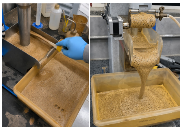
Figure 6: Niobium flotation – the more yellow colour reflects cleaner material
