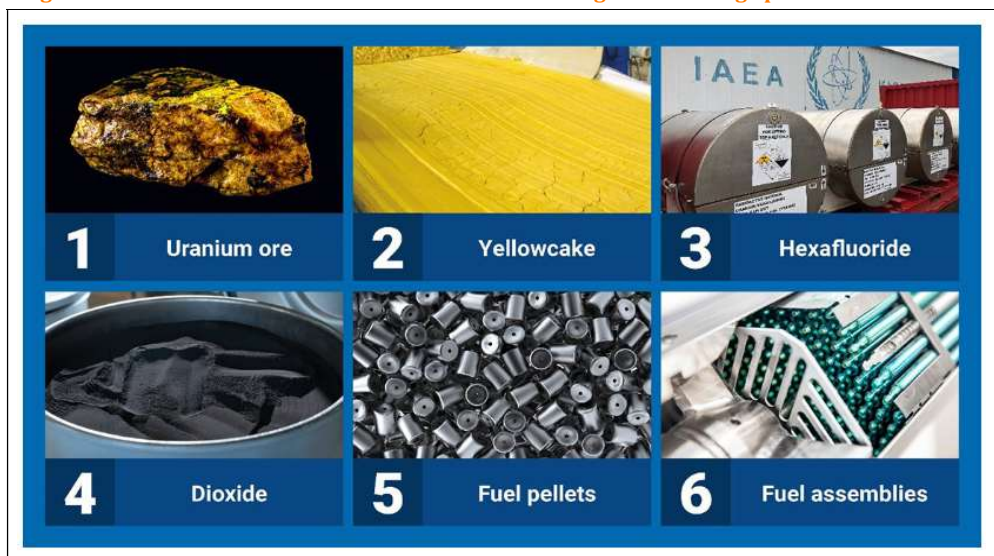
Figure 31: Uranium is converted into nuclear fuel through a multi-stage process
