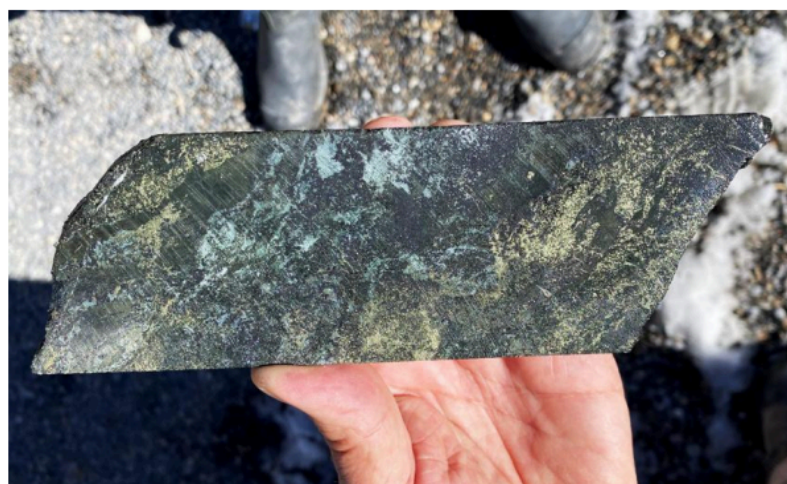
Figure 2: Cu-Au-Ag-In-Ga-rich mineralisation in WD22-01c
